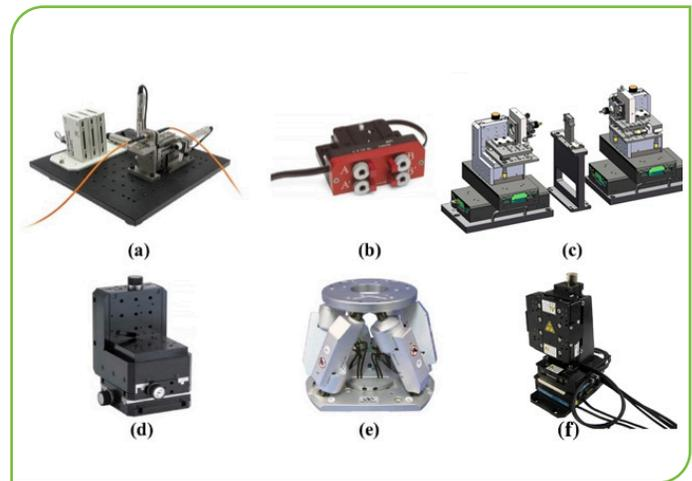
Figure 4. Manual and motorized motion stages: (a) Single fiber, single-end configuration with MKS 562 manual stages and CONEX-TRA actuators; (b) MKS 8071 4-axis aligner driven by Picomotor™ piezo actuators; (c) Double-sided configuration with MKS VP-25 and XMS stages; (d) MKS VP-25XA-XYZL integrated specifically for fiber alignment; (e) MKS HXP50 hexapod with horizontal and vertical beam paths; (f) MKS MLT-25XYZL/R integrated direct drive stages designed for fiber alignment.
