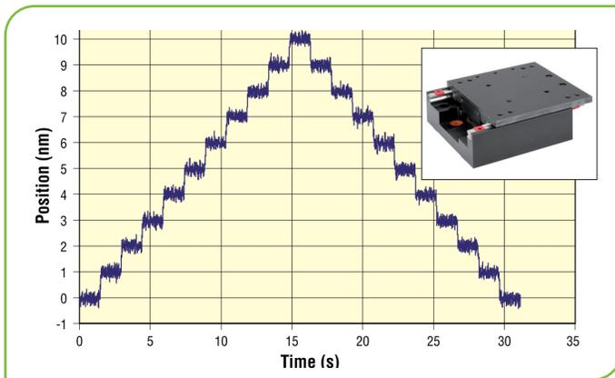
Figure 2. 1 nm MIM of an XMS linear stage;
