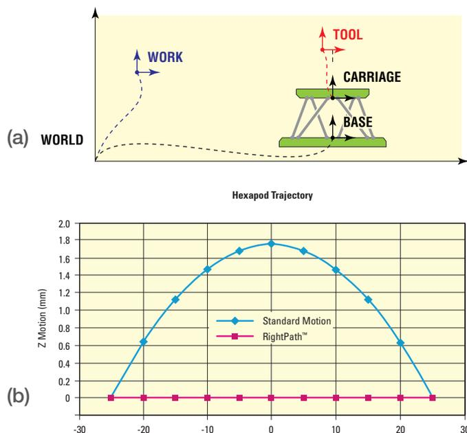
Figure 5. (a). MKS Instruments' HXP hexapod Work and Tool coordinate systems transformation of axes; (b) RightPath™ trajectory showing runout.
